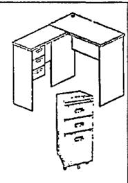
Main desk: "L - SHAPE" at least 25mm, thick HDF board with light gray HPL finish, post formed front with dark gray PVC/rabber edge sidings and inner grommet, panel legs with adjustable glider footings and 20mm, thick modesty panel.
