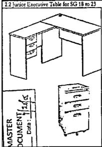
Main desk: "L - SHAPE" using at least 30mm, thick HDF board with light gray HPL finish, post formed front with dark gray PVC/rubber edge sidings and inner grommet, panel legs with adjustable glider footings and 20mm, thick modesty panel.
